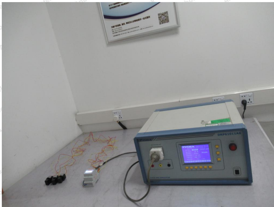
Photo of Voltage Dips and Interruptions Test
