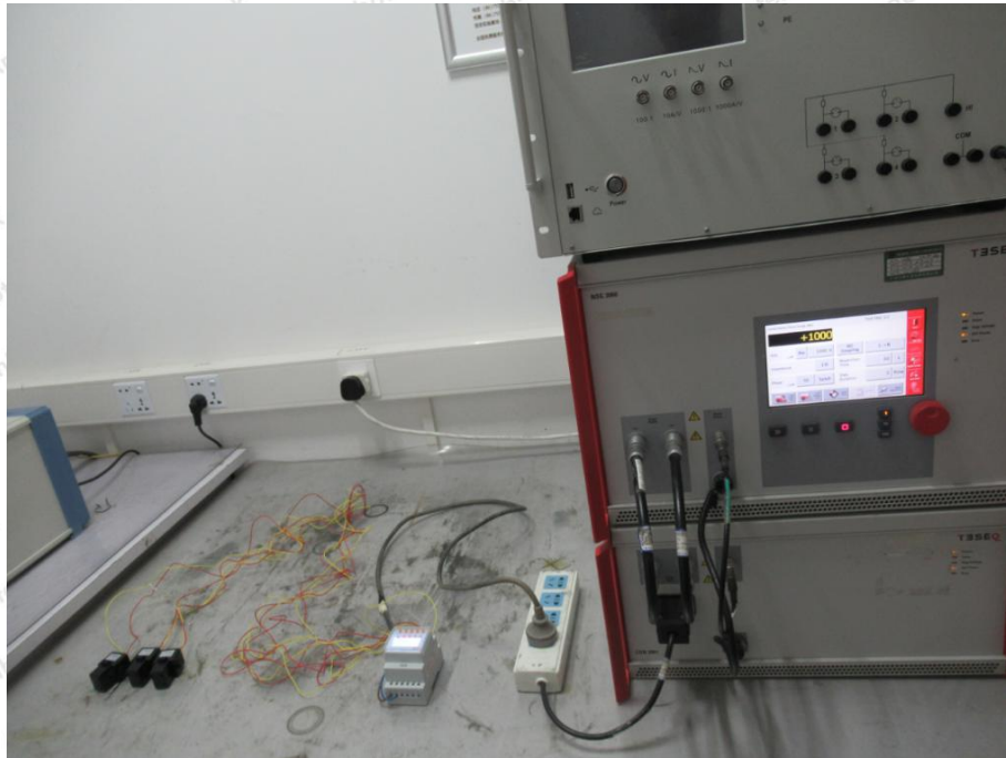
Photo of Surge Immunity Test
