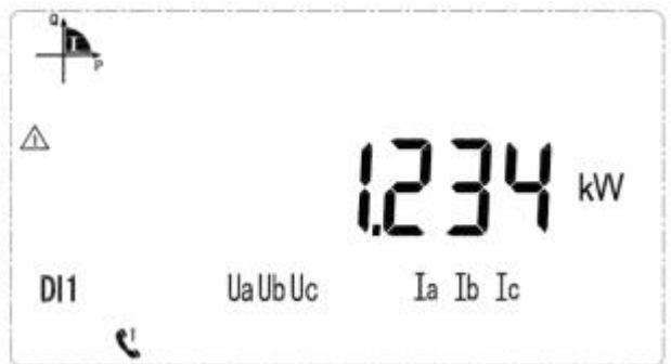
Current total power is 1.234kW
