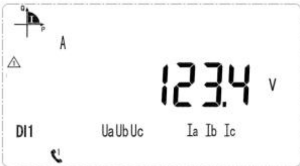
Voltage on A phase is 123.4V
