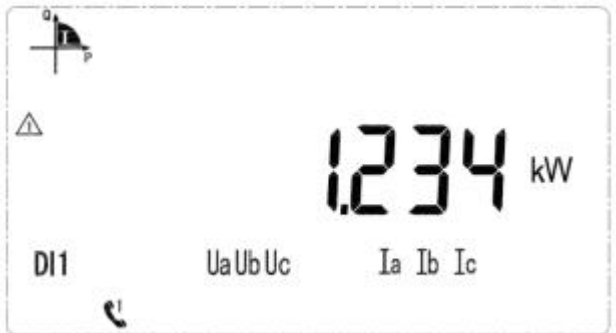
Current total power is 1.234kW
