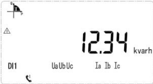
Current forward reactive energy 12.34kWh
