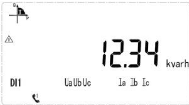
Current forward reactive energy 12.34kWh
