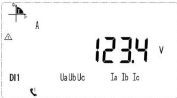
Voltage on A phase is 123.4V
