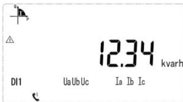
Current forward reactive energy 12.34kWh
