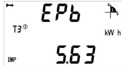
Current forward active energy on B phase
