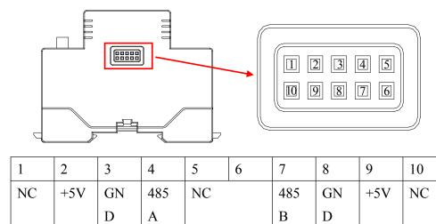
Note: The two interfaces of network port and terminal can only be used by one of the two (except for AWT100-CE), and cannot be used at the same time.
