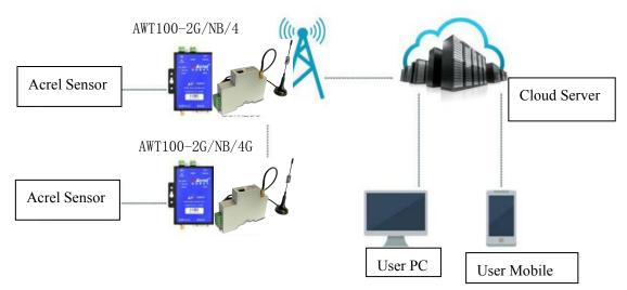
Figure 2 AWT100-2G/NB/4G Typical application of wireless communication terminal
