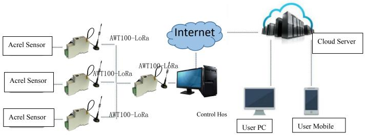
Figure 3 AWT100-LoRaTypical application of wireless communication terminal
