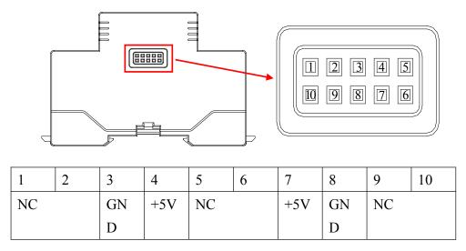
The side interface is used for the AWT100 wireless communication terminal to supply power through the AWT100-POW power module AC220V. The AWT100 wireless communication terminal is connected to the AWT100-POW power supply module through pins and fixed together by a buckle. The connection diagram is shown in Figure 4:
